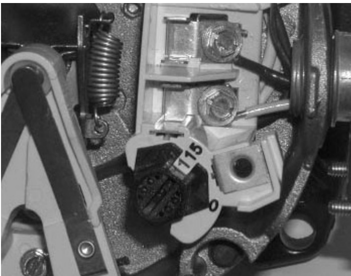
Figure 4: Motor Set for 115 Volt Operation
